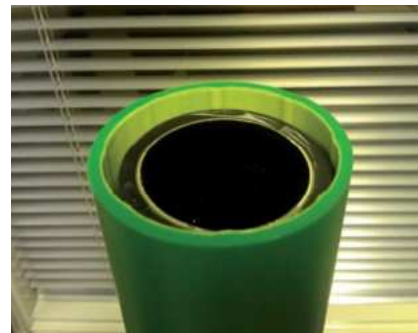
Picture 22: 4 layer fuel pipe with 3 layer protection pipe with ribs
