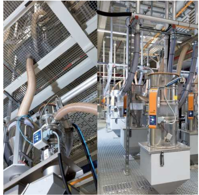
Material supply via the extruders with Metro G conveyor devices and intermediate containers above the machine level (Source: motan)
