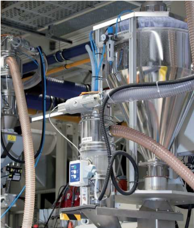
Precise solution for egeplast: Dosing and mixing system with Minicolor G dosing device and BTW hopper scale (Source: motan)
