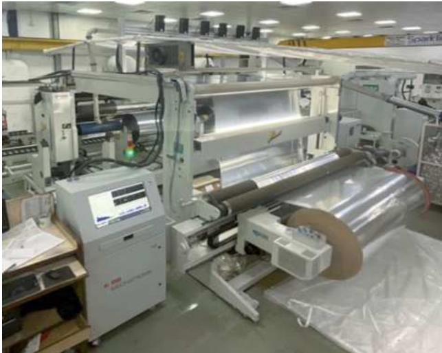
Picture 2: WIS-1000 System installed at a slitter-line
